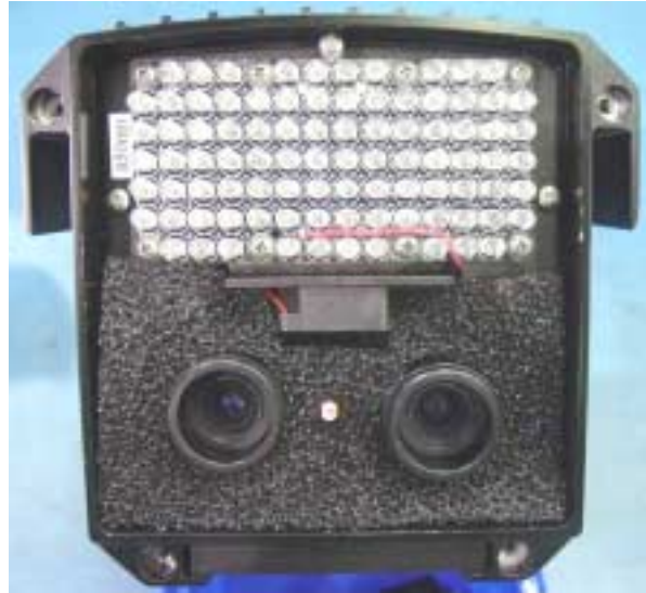
FIGURE 4 – 1 LED/Camera Lens Bracket Removal
