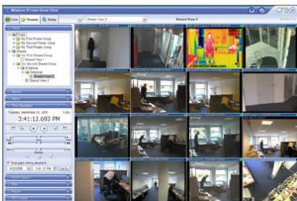
Example of the Smart Client , displaying images from 16 cameras
