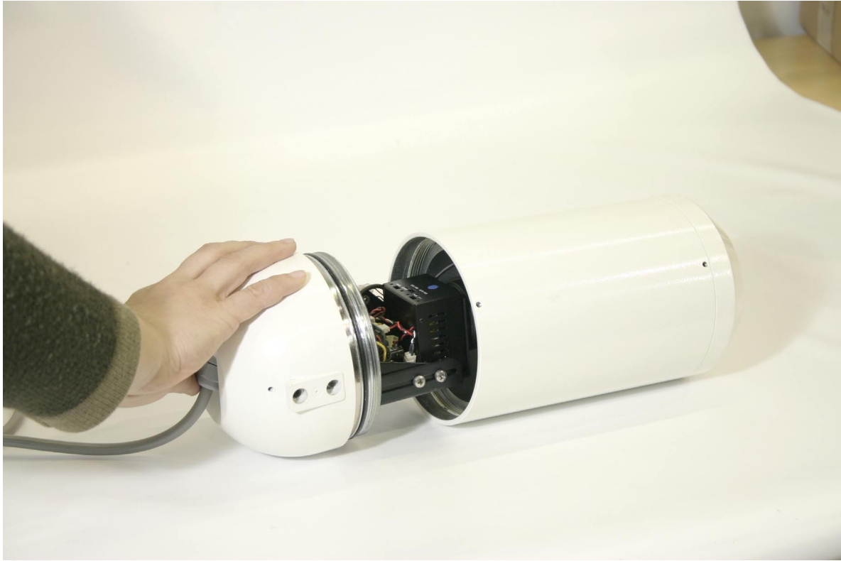
FIGURE 2 – 2 Rear Housing Removal From Main Enclosure
