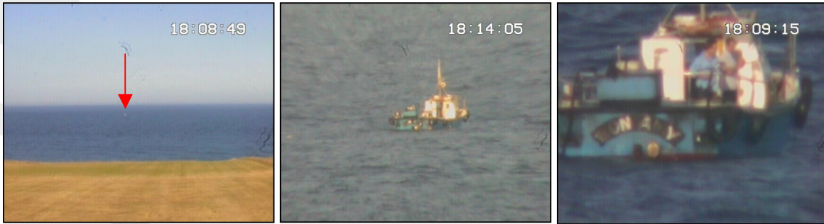
Above: The GVS1000 provides outstanding color daytime imaging. The 12.5mm to 750mm lens delivers 60x zoom for Recognition and Identification capabilities. The position of the vessel can be seen as a point of light and is indicated by the red arrow in the image at top left. Zooming in reveals two people on the deck of the "BON AMY". Range ~ 1km.
