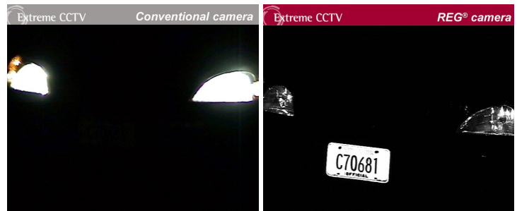
Overcoming the problems of headlight glare and low lighting, REG cameras deliver highly resolved license plate images in sub-zero temperatures.
